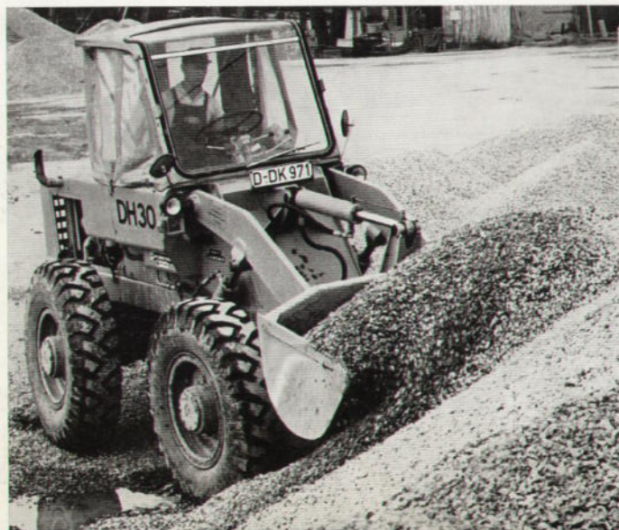
INTERNATIONAL Payloader DH-30 - 70 PS - 1,0 m³
