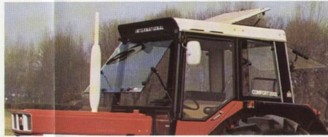
Windows and roof hatch are adjustable to admit fresh breezes.
